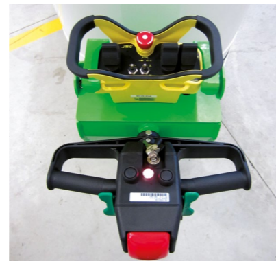
TILLER WITH RADIO REMOTE CONTROL (AS OPTION) FOR BOOM AND WINCH MOVEMENTS
